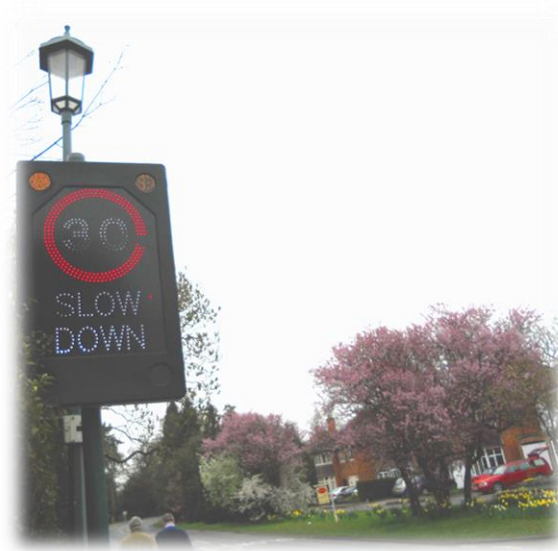
Vehicle activated ‘Slow down’ sign in Hampton-in-Arden
